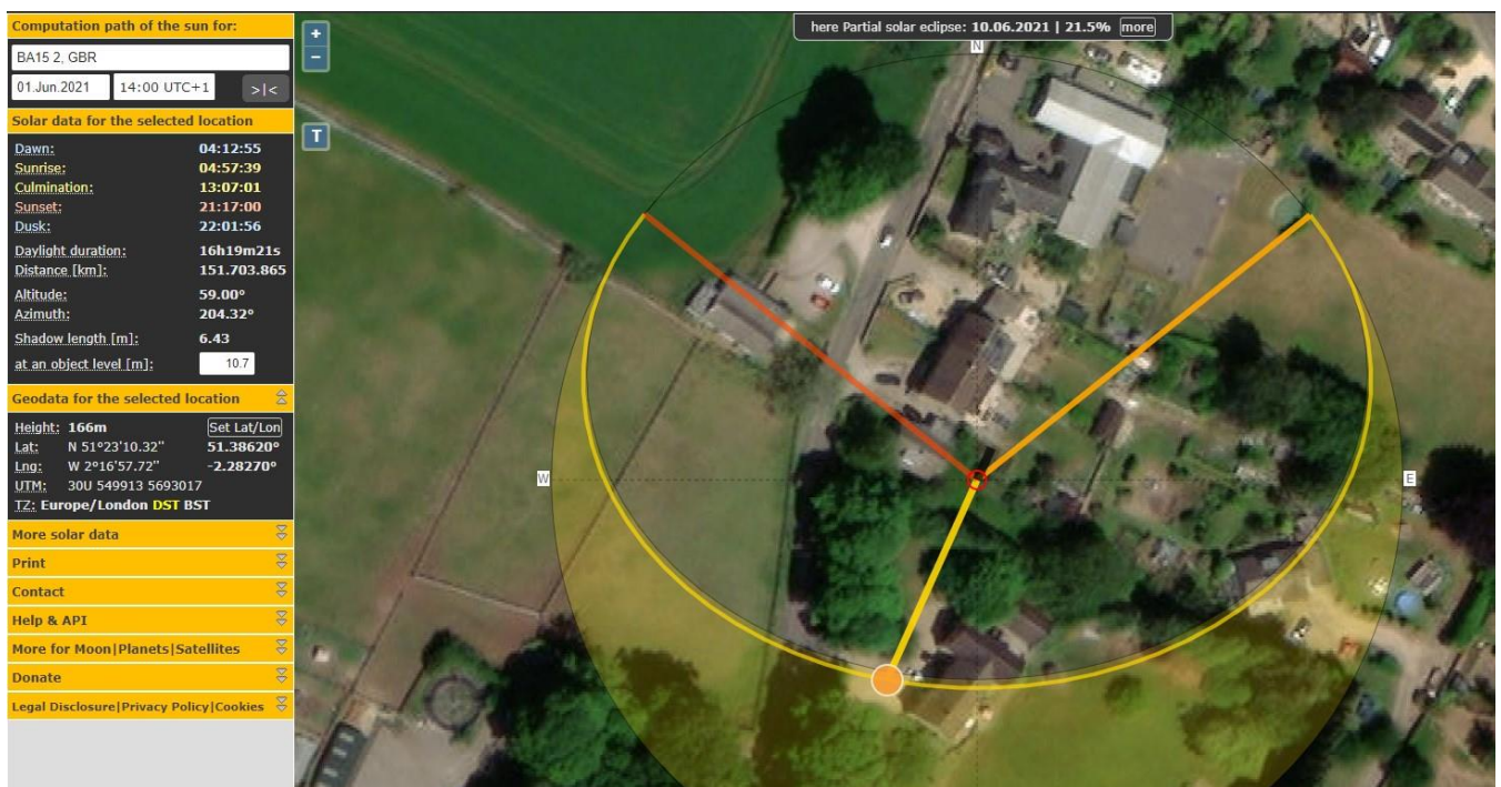
Above: Sun calculation for the proposed replacement property as of 1 June (2pm)
